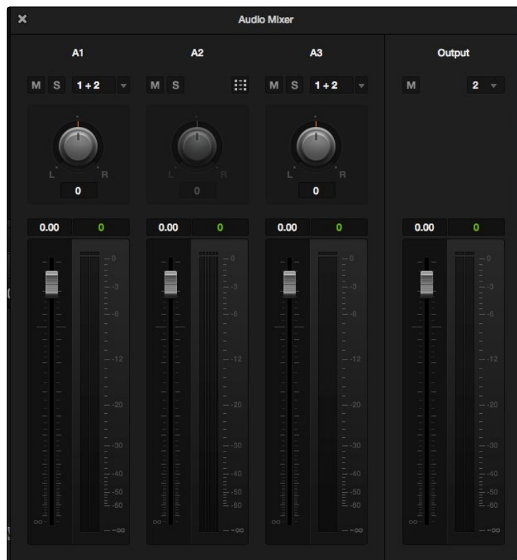
The Audio Mixer, with three channel strips corresponding to the three tracks in the timeline
