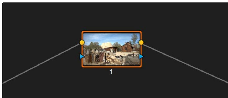
A single node, the RGB and KEY inputs and outputs are clearly visible
