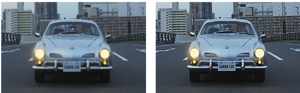
Before - The original image, After - Sharpening applied to only the Y' channel of the image
