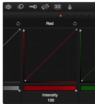
Controls attached to each Custom curve; the handle on the upper-right hand side is the YSFX vertical slider, and the slider underneath is the Curve Mix slider
