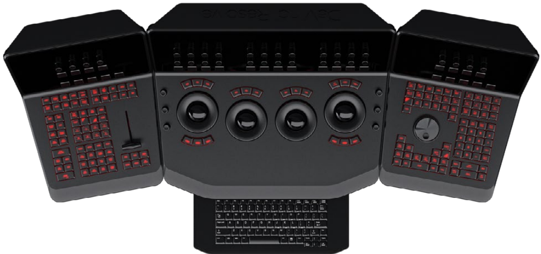
The Trackball panel includes a slide-out keyboard
