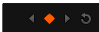
The three keyframe controls that appear in the Inspector, from left to right: Previous keyframe, Create/Delete keyframe, Next keyframe
