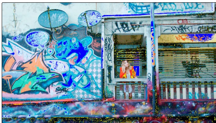
Areas of the image that violate broadcast safe are highlighted in blue
