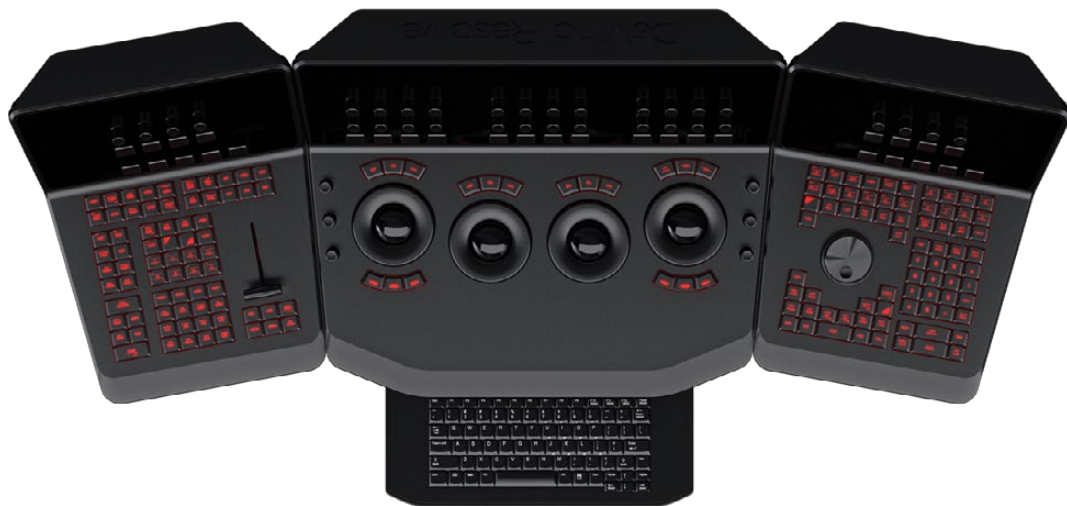
The Trackball panel includes a slide-out keyboard
