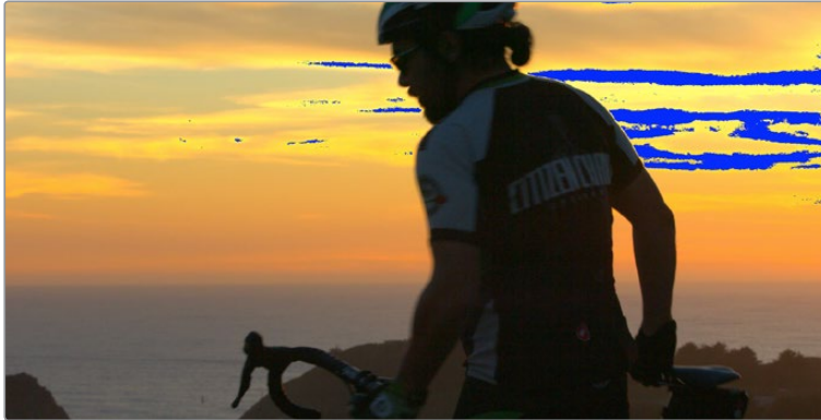
Areas of the image that violate broadcast safe are highlighted in blue
