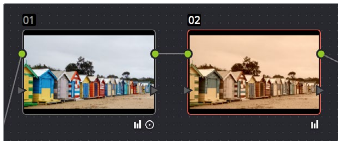
Choosing your battles—the image coming out of Node 1 will be easier to key than the highly stylized image coming out of Node 2
