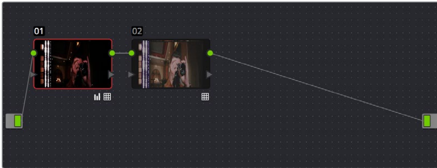
Using three nodes to convert a film scan using LUTs, node 1 converts from Negative or Print to Linear, node 2 converts from Linear to Rec. 709, and node 3, if required, inverts the color
