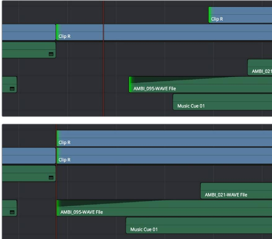
Before and After a multi-track extend edit performed in Trim mode; you can see that the lowest numbered track with a selection defines how far the Timeline will be rippled
