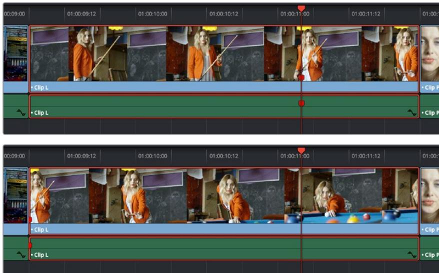
Using the Extend edit to Slip a clip in the Timeline, the red marker shows that the frame at the playhead is slipped back to the In point of that clip in the Timeline
