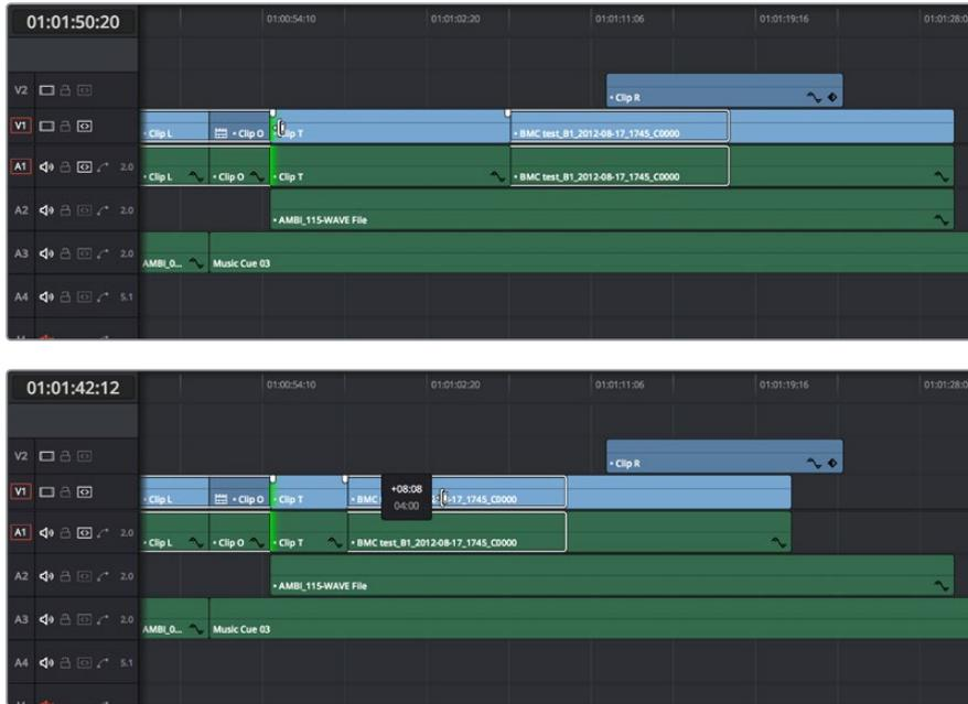
Before and After, clip to the right of Clip T on tracks V1 and A1 are rippling because those tracks' Auto Select controls are enabled, but clips on tracks V2 and A2 aren't rippling because those tracks' Auto Select controls are disabled
