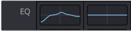
The channel strip's EQ indicator, (Left) EQ is adjusted, (Right) EQ is detente
