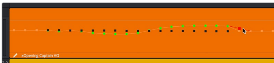
Black points show the previous levels when samples have been edited in a clip
