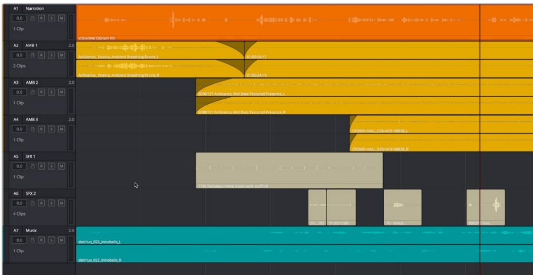
(Top) Stereo audio in the Edit page represented by a single track (Right) The same stereo audio in the Fairlight page shows the two lanes that correspond to each of the stereo audio tracks
