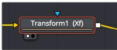
Viewer assignment buttons at the bottom left of nodes indicate when they're being viewed, and which dot is highlighted indicates which viewer that node is loaded into
