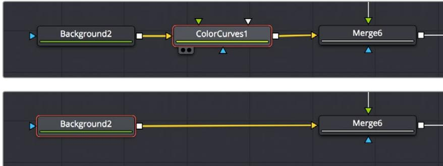
(Top) Before deleting a node from a node tree, (Bottom) After, upstream and downstream nodes have automatically reconnected
