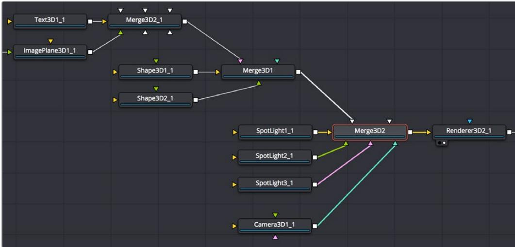
An example of a 3D scene using multiple Merge3D nodes that are working together; the upstream Merge3D nodes arrange the 3D objects placed within the scene, while the last Merge3D node (orange) lights and frames the scene
