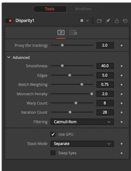
The Disparity node analyzes a stereo pair of images and generates an X&Y disparity map
