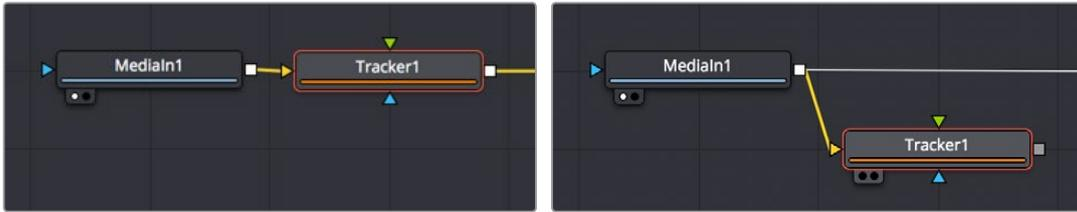
(Left) Tracker node connected serially so it can both track and transform the input image, (Right) Tracker connected as a branch to indicate it only contains tracking data, without using it directly
