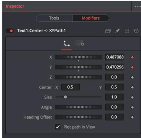
XY Path modifier controls in the Modifier tab of the Control panel
