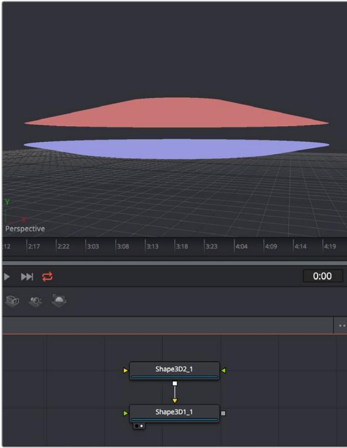
Connecting one Shape3D node to another directly to combine them, transforming the last downstream 3D object also transforms all upstream objects; the last Shape3D node is viewed, showing both
