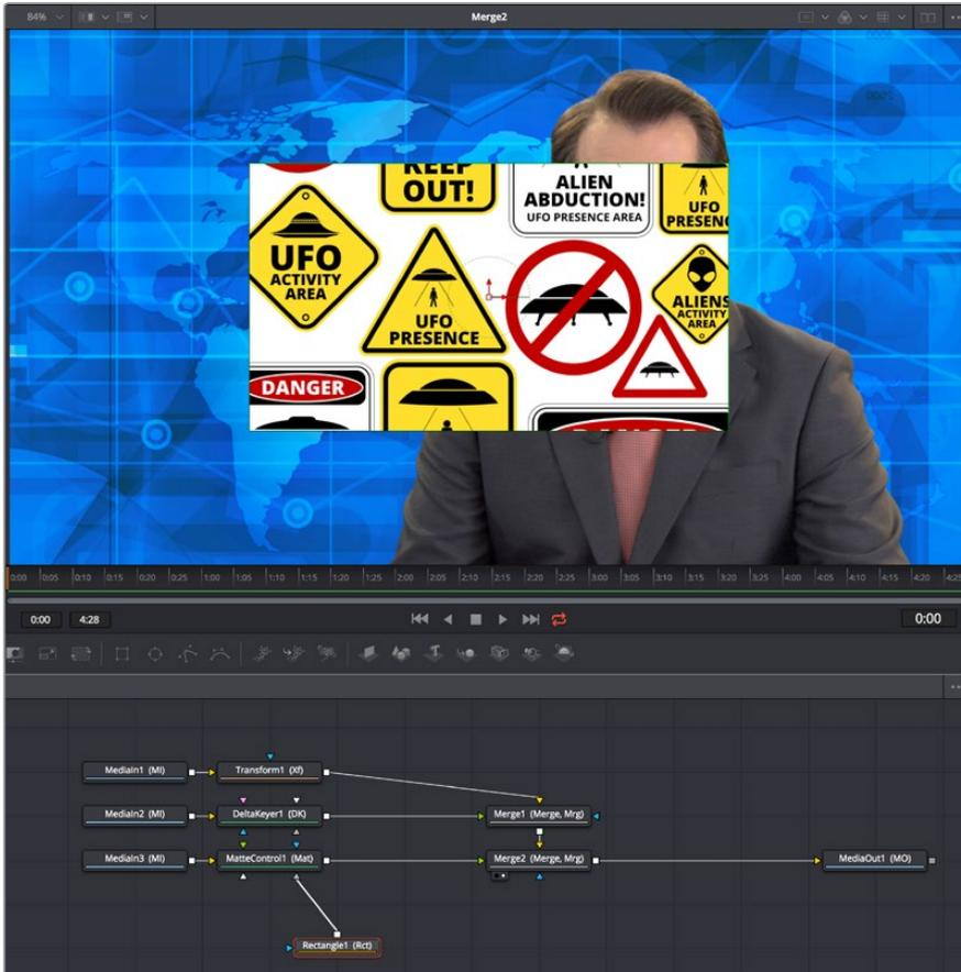
Masking the logo using a Rectangle mask connected to a MatteControl node
