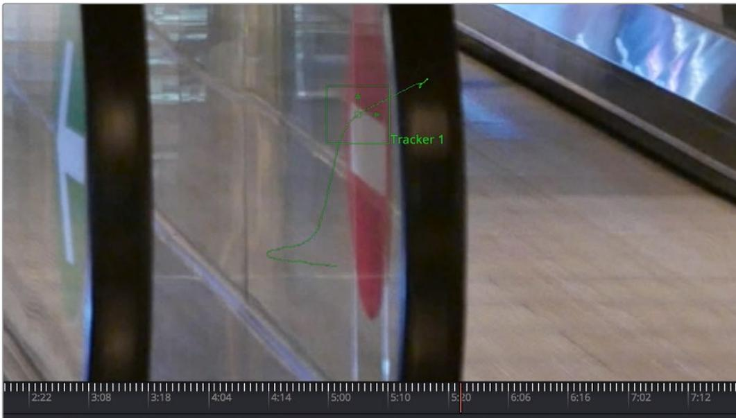
A motion path that indicates the tracked motion path, and tic marks indicate tracking data keyframes
