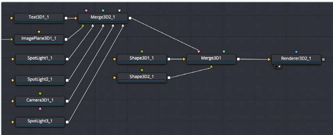
You can build elaborate scenes using multiple Merge3D nodes connected together
