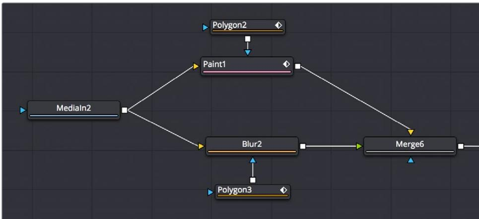
A MediaIn node branched to two node operations and then recombined using a Merge node
