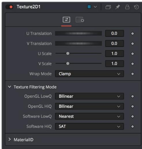
The Texture2D node is used to translate a texture in the UV space of the object, as well as set the filtering and wrap mode
