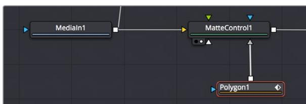
Feeding a Polygon node to a MatteControl node to do rotoscoping
