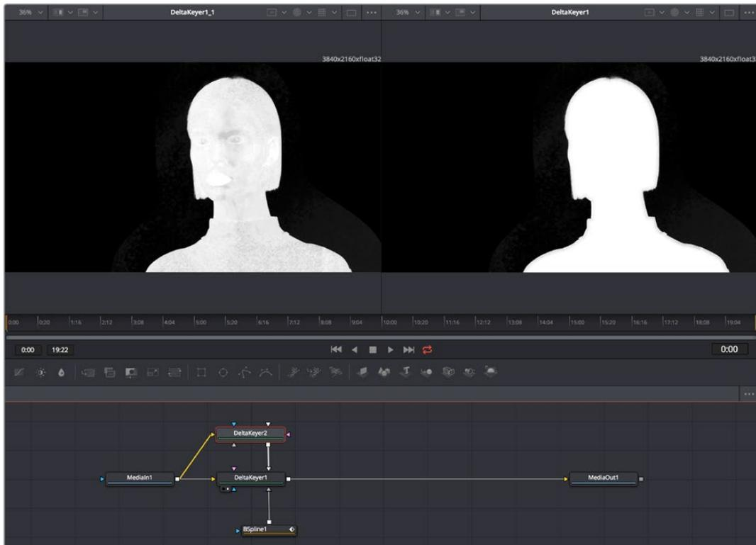
Filling in holes in the mask pulled by the DeltaKeyer1 node (at left) with another, harder but eroded key in DeltaKeyer2 that's connected to the SolidMatte input of DeltaKeyer1.
