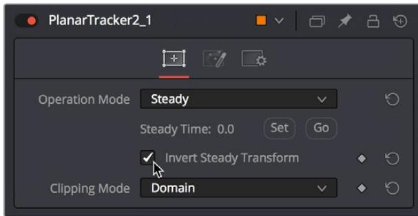
Turning on Invert Steady Transform to try and put the image back to the way it was
