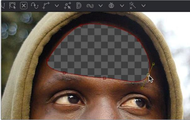
Drawing a shape to isolate the forehead gives an inverted result at first when using the Garbage Matte input of the MatteControl node to attach the Polygon to the MatteControl node
