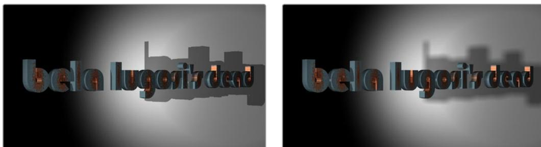
(Left) When the Renderer3D node "Renderer Type" pop-up is set to OpenGL Renderer, you cannot render soft shadows or excessively large textures, (Right) When the Renderer3D node "Renderer Type" pop-up is set to Software Renderer, you can render higher quality textures and soft shadows
