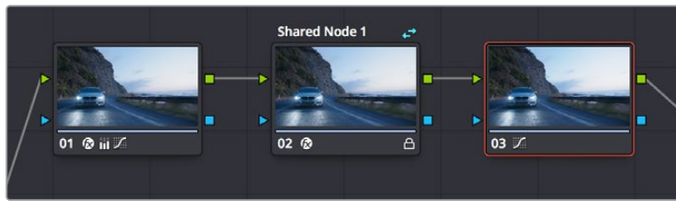
A grade with an Unshared (at left) and Shared node (at right), a badge indicates the Shared node, which is also locked
