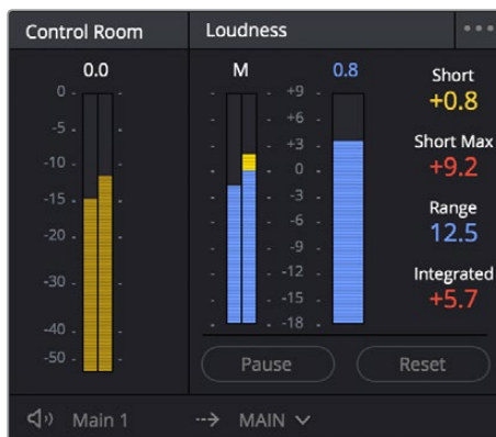
The Control Room meters (at left), and Loudness meters (at right)
