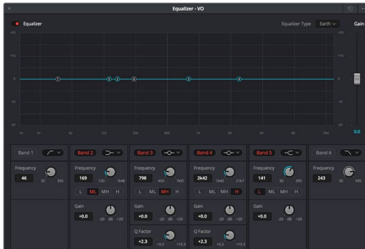
The 6 Band parametric equalizer that can be applied to every track
