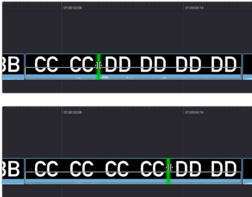
(Top) Clicking an edit between clips CC and DD, (Bottom) Dragging to the right rolls it forward, simultaneously resizing clips CC and DD
