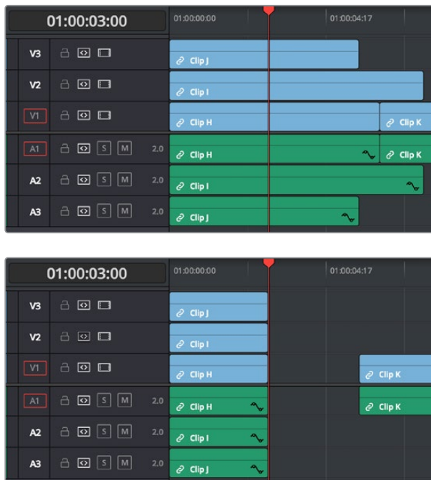
Trimming all clips at the position of the playhead
