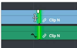
Selecting incoming or outgoing halves of an edit point to resize or ripple
