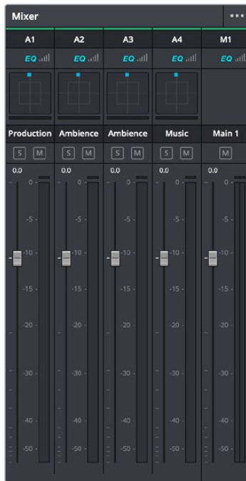
The Audio Mixer, with four channel strips corresponding to the four tracks in the Timeline
