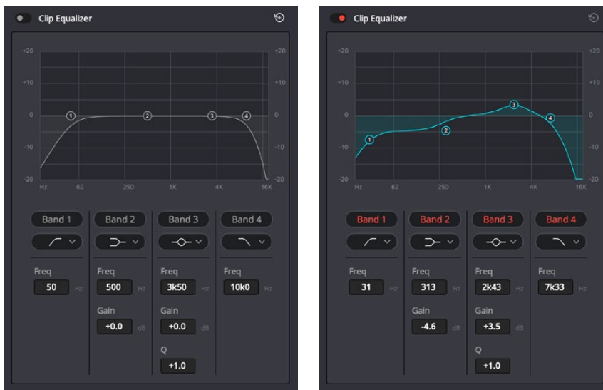
The channel strip's EQ indicator, (Left) EQ is at detent, (Right) EQ is adjusted
