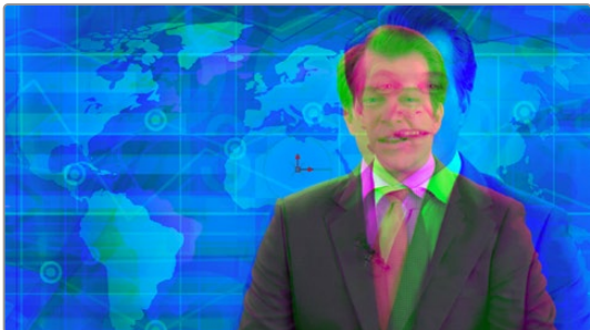
Transforming only the green color channel of the image with a Transform effect.
