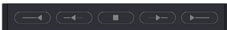
The analysis buttons, left to right: Track from Last Frame, Track Backward, Stop Tracking, Track Forward, Track from First Frame.
