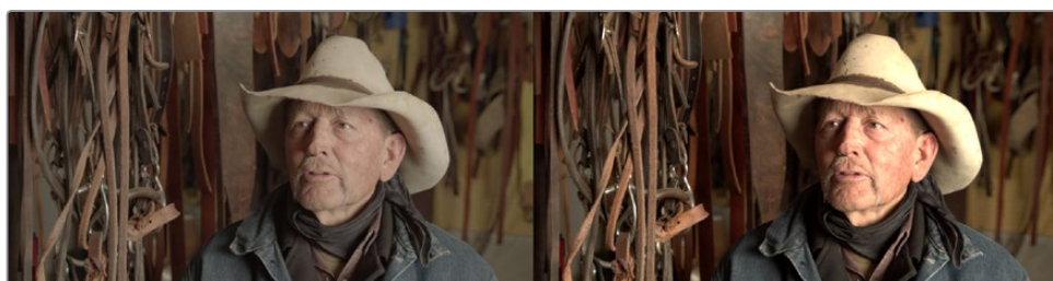
A clip displayed with a nonlinear, log gamma curve (left) and corrected in the viewer using a LUT (right).
