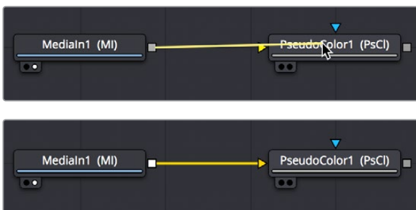
Side by side, dropping a connection on a node’s body to connect to that node’s primary input.
