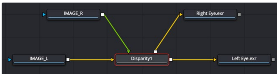
Left and right eye images are connected into a Disparity node to generate and render out a stereo image
