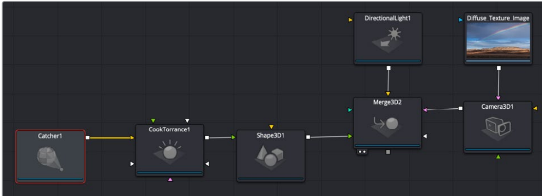
A Catcher node output is connected to the input of the geometry node that receives the texture projection
