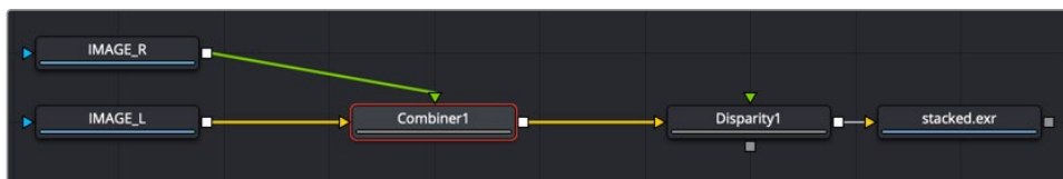
Left and right eye images are connected into a Combiner node to generate a stacked stereo image
