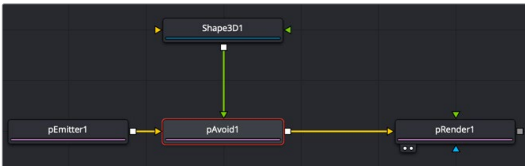
A pAvoid node using a Shape 3D node as the region to avoid
