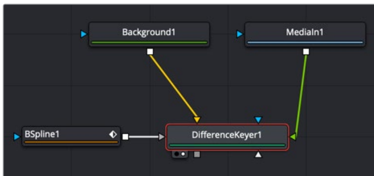
A Difference Keyer with two inputs: one of the subject on a background and the other of just the background
