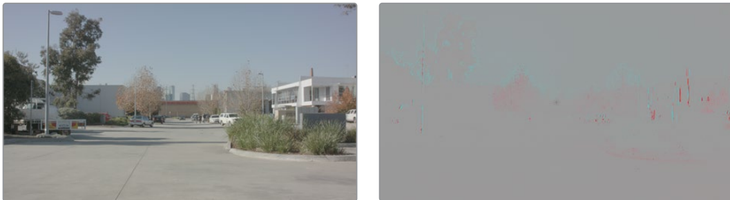
(Left) The original image in close up, showing chromatic aberration, (Right) The image with Estimated Red Fringes enabled, letting you see the specific problems as differences between red and cyan stripes
