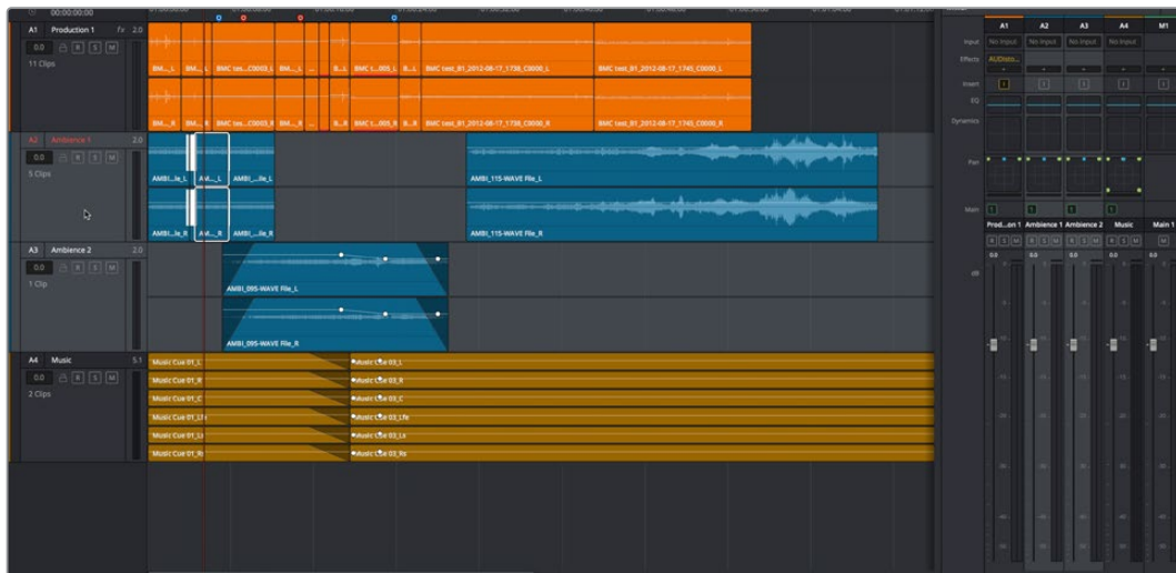
Selecting multiple channel strips results in the selection of multiple tracks
