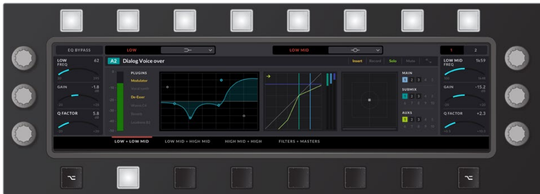
Editor screen displaying EQ processing controls assigned to adjacent soft buttons and knobs
