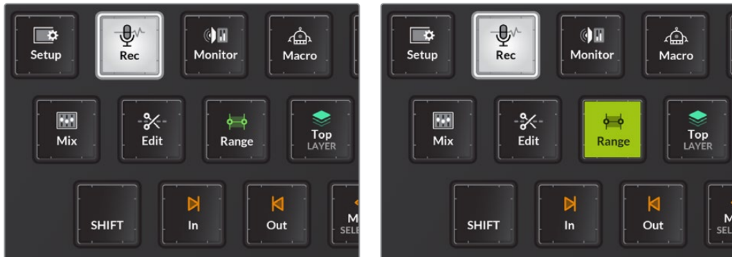
Range key unlatched and Range key latched
