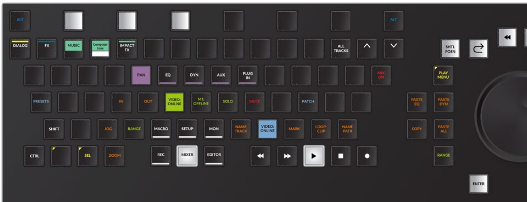
Alternate Mixer toolset with Mix On unlatched, Copy/Paste latched, and Copy/Paste keys available near the jog wheel
