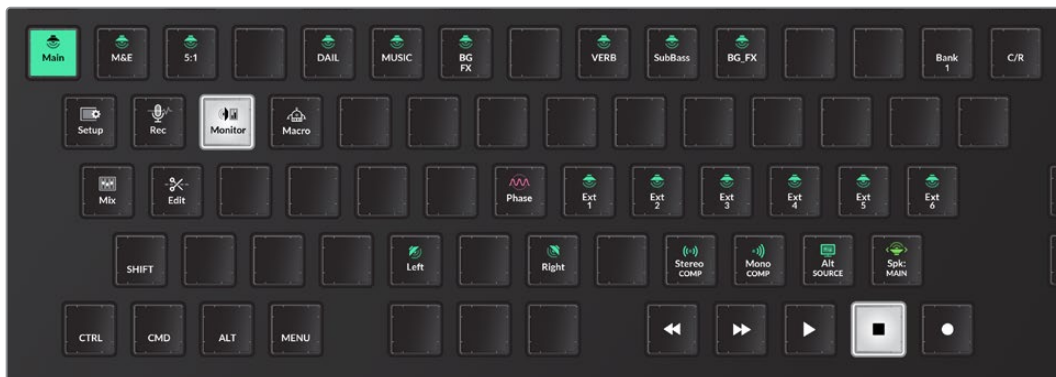
Monitor mode default keys showing Control Room monitoring
