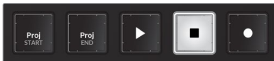
Transport keys with Control modifier engaged to reveal Project Start and Project End keys
