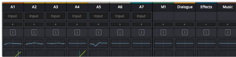
The Audio Mixer is divided into two sections, one for tracks (at left) and one for buses (at right)
