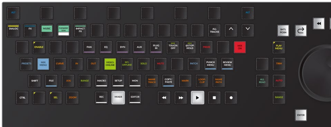
Alternate Mixer toolset with Mix On latched and Mix automation keys available near the jog wheel
