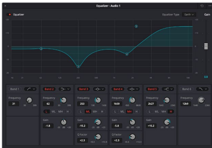
DaVinci Resolve Fairlight interface displaying EQ window that can be opened and closed with a long-press on the EQ key
