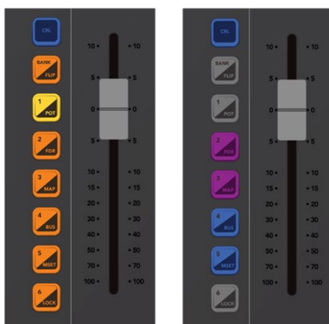
Fader Bank display buttons and touch-sensitive fader with Bank 1 selected, and with the secondary button functions available while the Control button is pressed.
