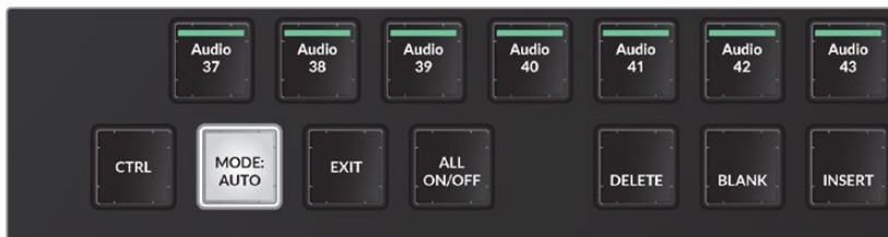
Manual Fader Bank mapping action keys in the bottom row of the picture keyboard
