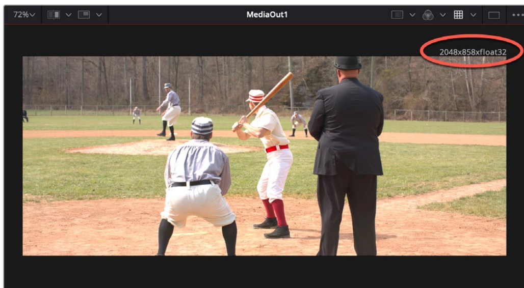
The available resolution and bit depth of the currently selected clip is visible above the upper right-hand corner of the Viewer, circled in red
