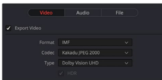
The Video Settings to use for creating a Dolby Vision IMF in the Deliver page
