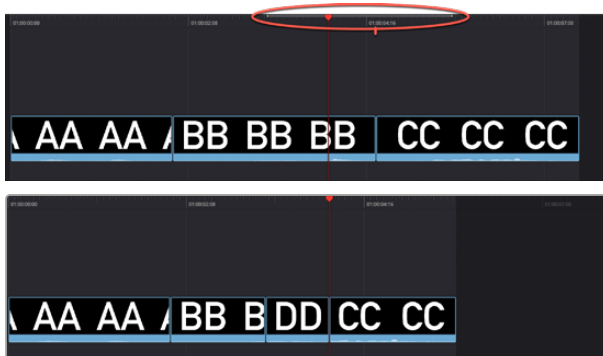
Performing a Ripple Overwrite to substitute a In/Out range of the Timeline (part of clips BB and CC) with the incoming clip DD
