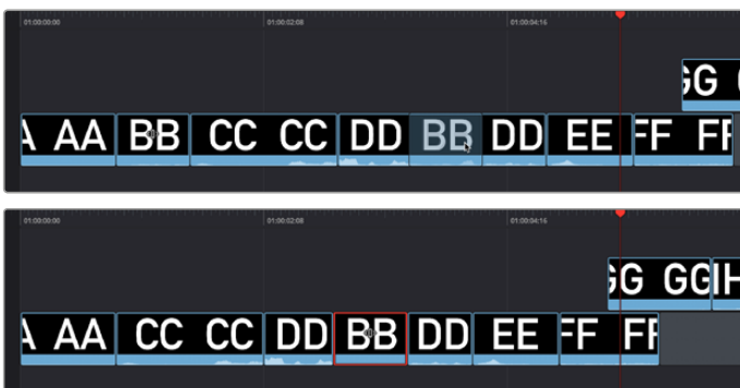
(Top) Dragging clip CC to partially overlap clip DD in order to overwrite it, (Bottom) After dropping clip CC to partially overwrite the beginning of clip DD, clip DD is shortened and the other clips in the Timeline move left to fill the gap in Track 1
