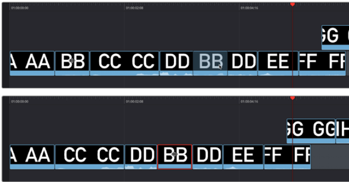
(Top) Dragging clip BB and pausing to overwrite part of clip DD, (Bottom) Clip BB is moved, overwriting the middle of clip DD which is now in two pieces; the rest of the Timeline moves left to fill the gap left by moving clip BB in Track 1
