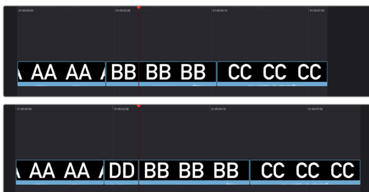
(Top) Before doing a Smart Insert, (Bottom) After inserting clip DD between clips AA and BB
