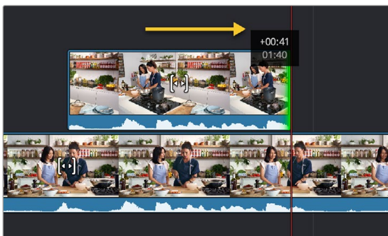
Performing a Live Overwrite by holding down the Camera 5 key and rotating the search dial to the right
