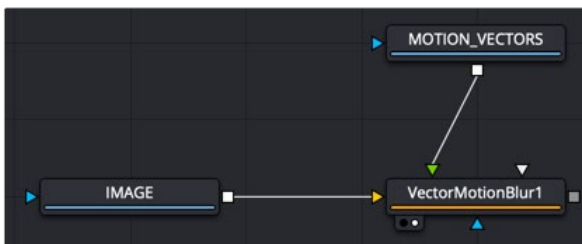
A Vector Motion Blur node applied to a MediaIn or Loader node with motion vectors connected to the Vectors input
