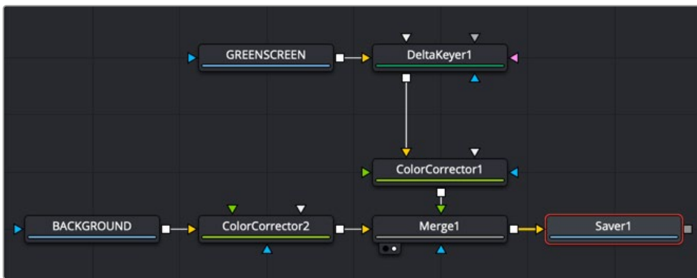
Saver node added to the end of a node tree to render the composition
