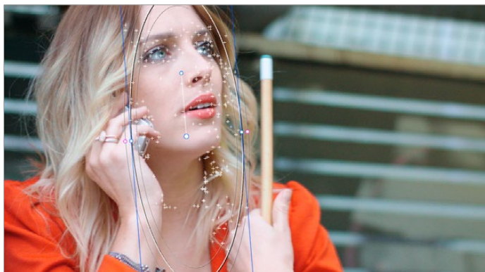
Object tracking in progress. Tracking points are automatically placed over trackable features of the image
