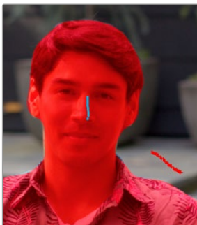
Blue strokes identify a person or feature to isolate, while red strokes identify things that shouldn't be included in the mask.
