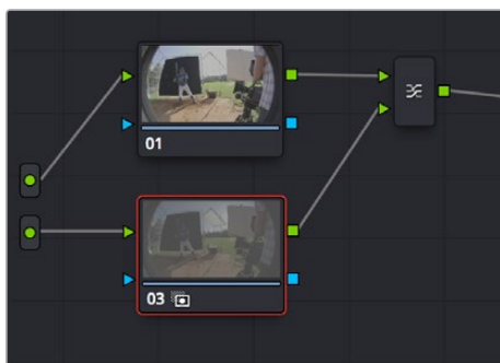
A node tree that uses a Layer Mixer node to mix two Corrector nodes, each connected to separate outputs for the regular and highlight exposures
