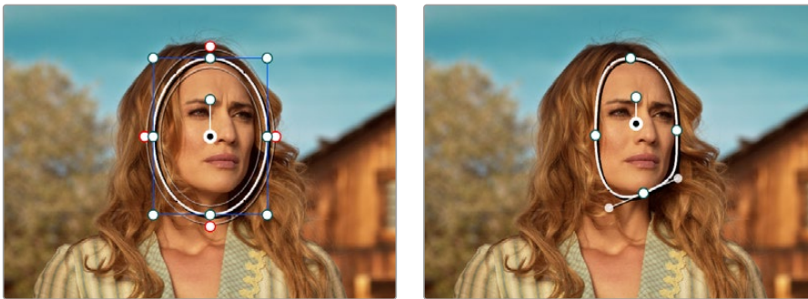
Before and after converting a circular window to a Bezier curve and adjusting the result, before adding softness to the edge
