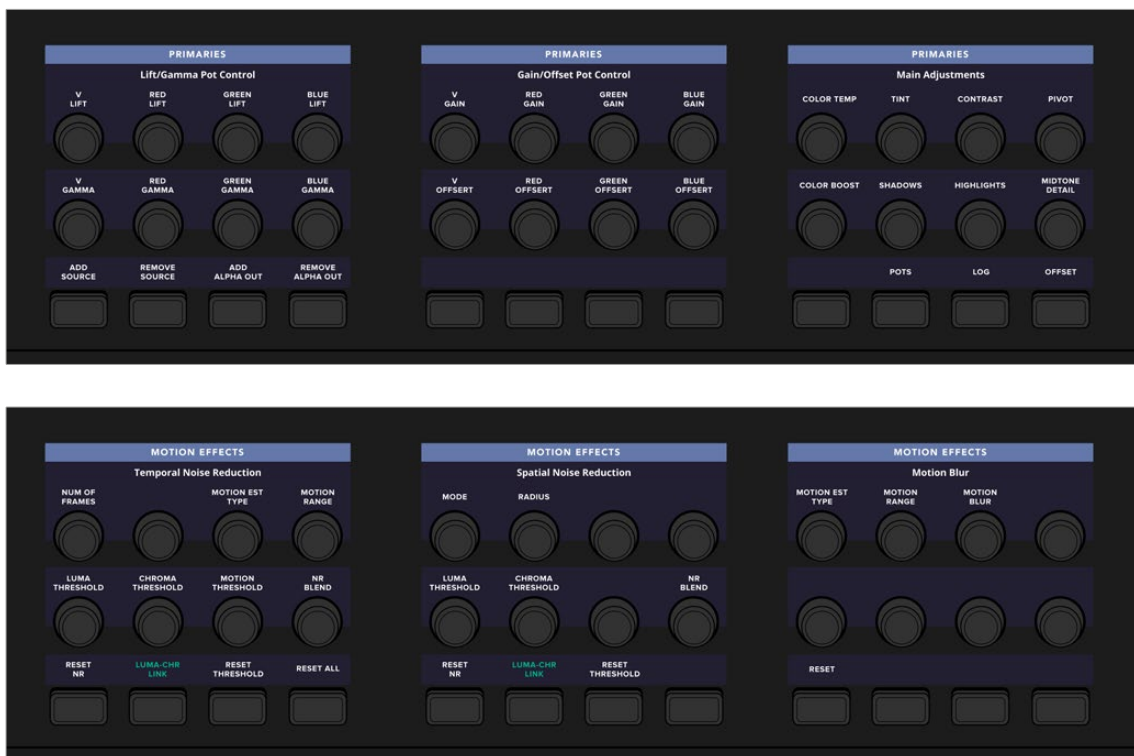
(Top) The Trackball panel's soft menu controls corresponding to the Primaries palette, (Bottom) the soft menu controls corresponding to the Motion Effects palette; note how all the controls update to be contextual to the palette that's currently in use
