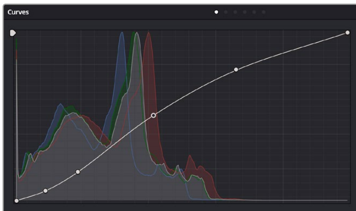
The histogram appearing underneath the Custom Curves shows a YRGB histogram analysis
