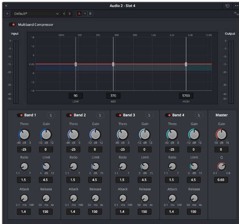
The default setting of the Multiband Compressor
