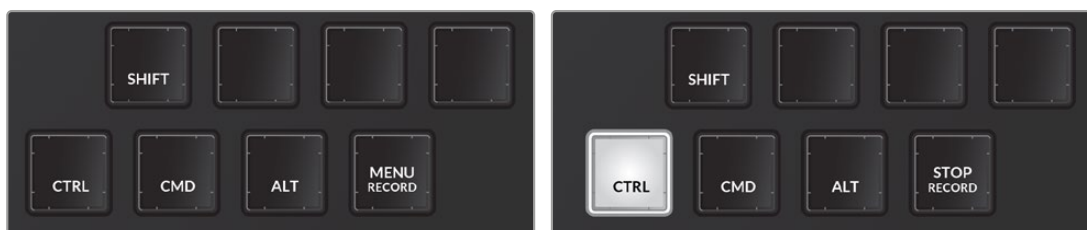
Menu becomes Menu Record key during macro recording and Stop Record when Control key is pressed during macro recording
