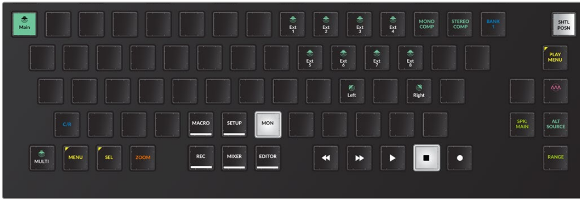
Alternate Monitor toolset with Phase, Main/Near Speaker selection, and Alt Source keys available near the jog wheel
