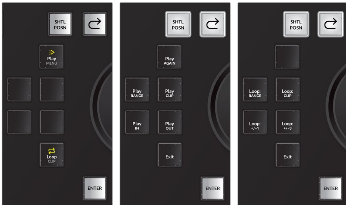
(Left) Default soft menu keys with Play Menu key unlatched with Loop key set to Loop Clip, (Center) Play Menu key latched, showing Playback Options keys, (Right) Loop key latched, showing Loop Options menu for assigning Loop Playback mode
