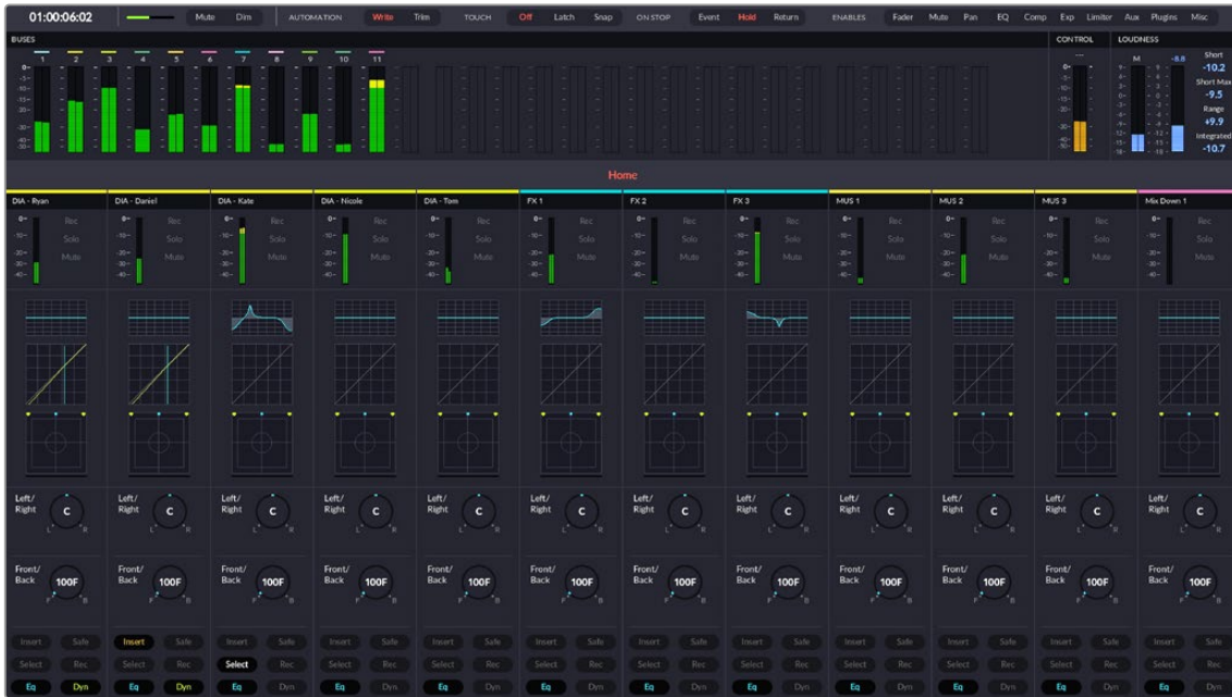
Optional HDMI monitor displaying Strip mode layout with an identical set of parameters in-line with each of the 12 channel strips, including from the top down: Track color, Name, Level, Status, EQ, Dynamics, Panning controls, and Channel Extension buttons.
