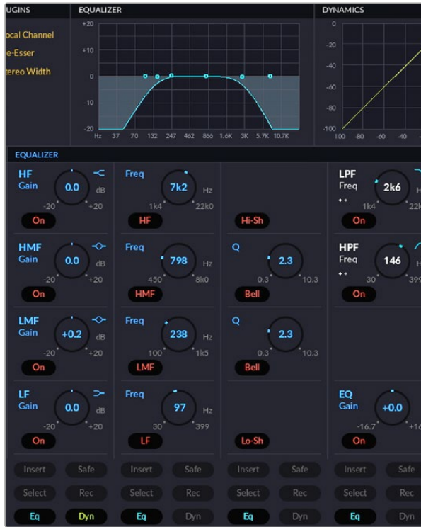
EQ control set visual feedback in optional HDMI monitor
