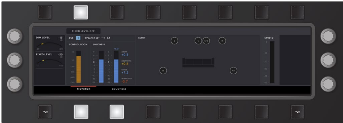
Monitoring mode layout with visual feedback for Dim and Fixed levels, Control Room, Loudness, and Studio meters, as well as a graphical representation of the speaker configuration and listening environment.
