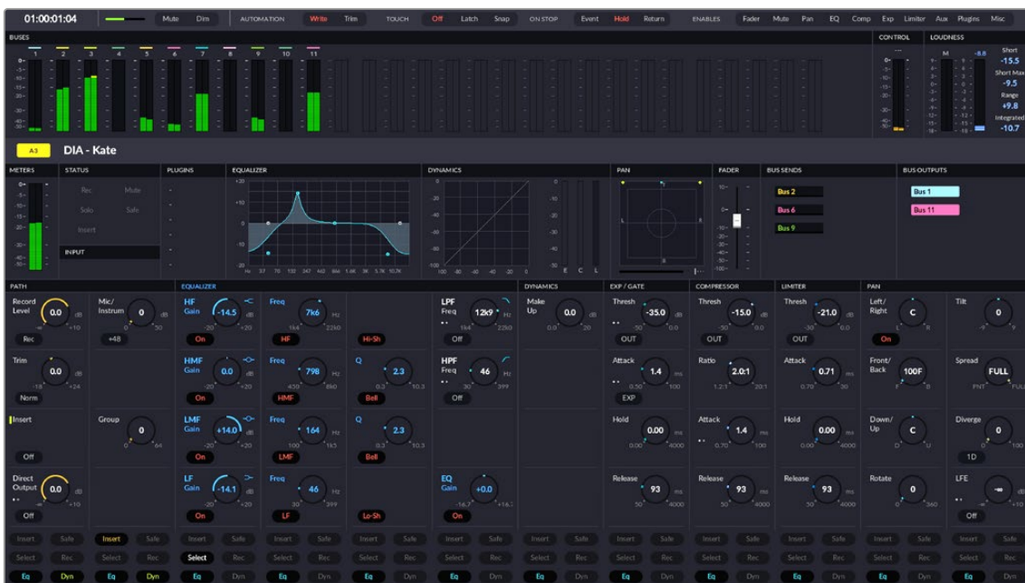
Optional HDMI monitor displaying the Channel Control mode layout, which includes 192 different parameters for the active channel. Parameter controls currently mapped to the LCD displays, knobs, and SEL buttons are highlighted with blue text.
