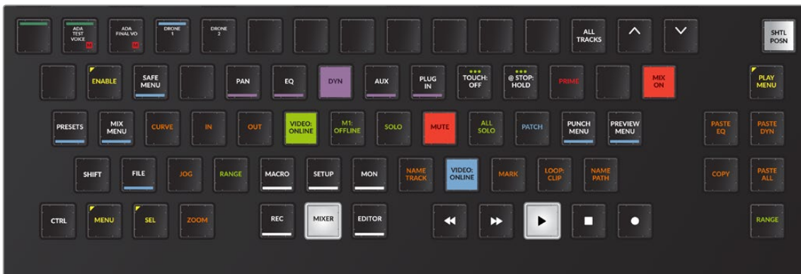
Alternate Mixer toolset with Mix On latched and Mix automation keys available near the jog wheel
