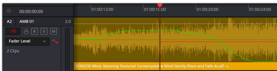
Setting new levels to overwrite previously recorded automation displays a red line
