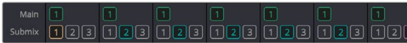
Main and Submix buttons let you assign tracks to buses, and buses to other buses
