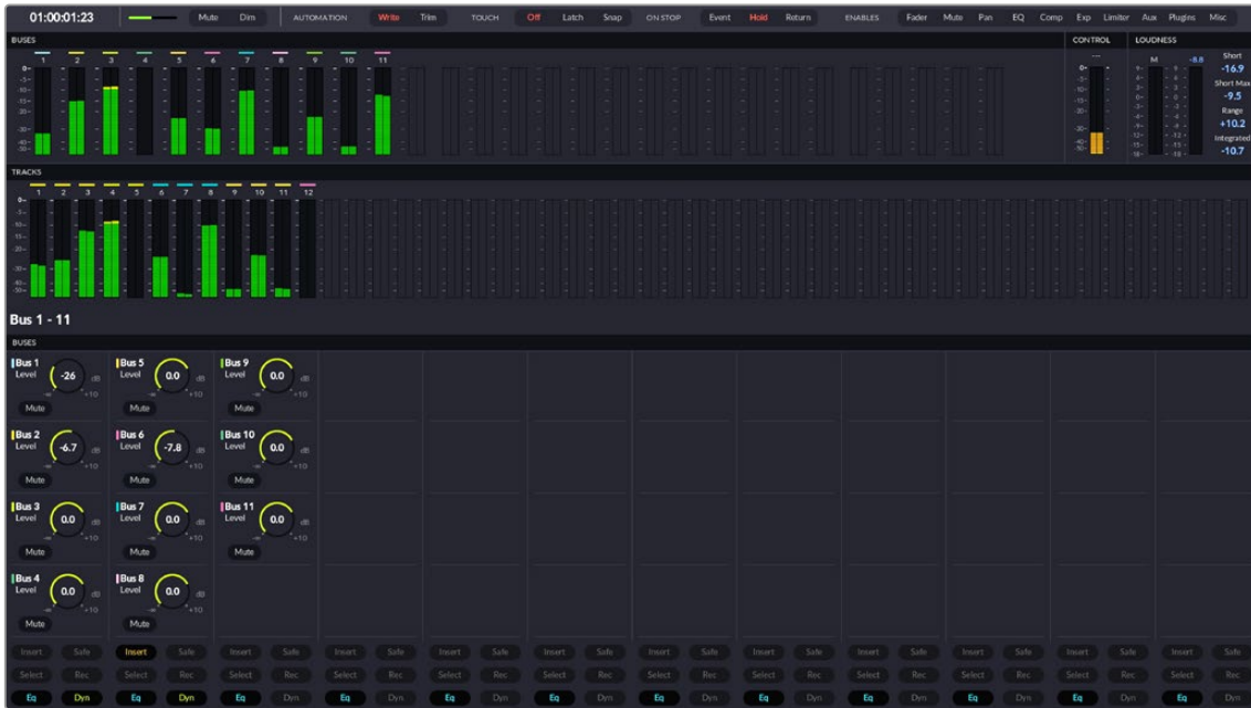
Optional HDMI monitor displaying the Master Control mode layout with bus meters, level, and mute for each of the master buses.
