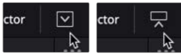
(Left) The button for expanding a panel to full height, (Right) The button for contracting a panel to half height
