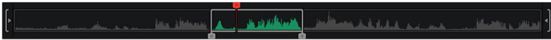
Defining a range of media in the Viewer using In and Out points
