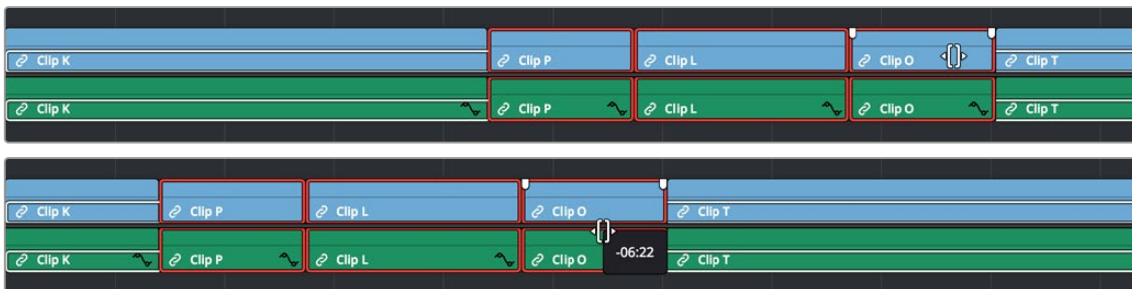
(Before) Selecting four clips to slide, (After) All four clips slid to the right using the mouse
