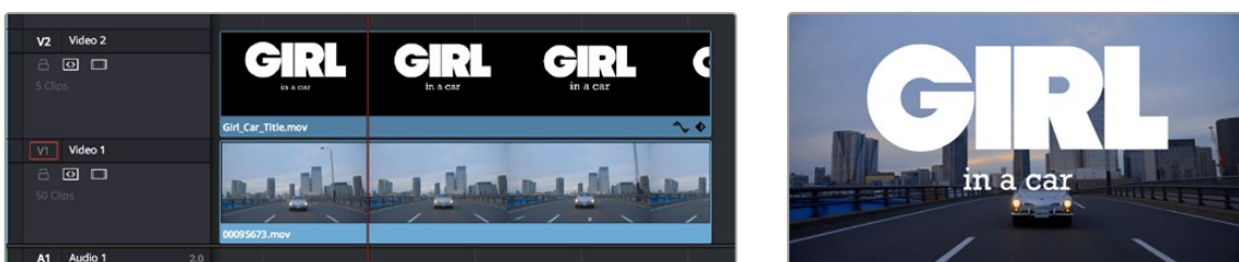
Superimposing a clip with an alpha channel above automatically composites that clip against the clip beneath it
