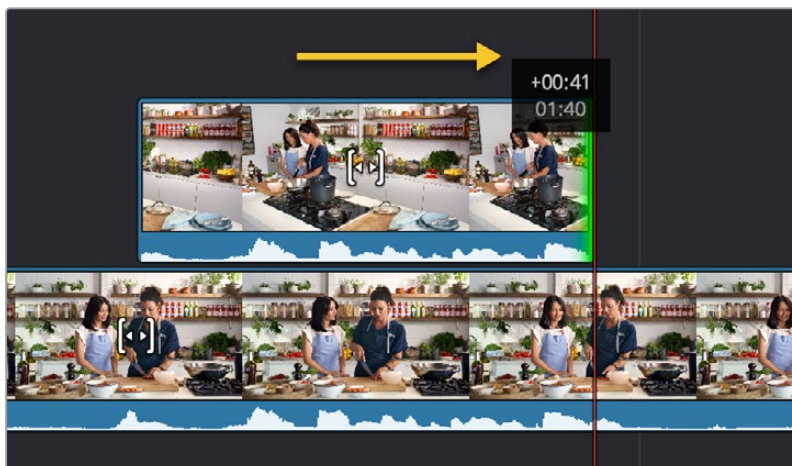
Performing a Live Overwrite by holding down the Camera 5 key and rotating the search dial to the right
