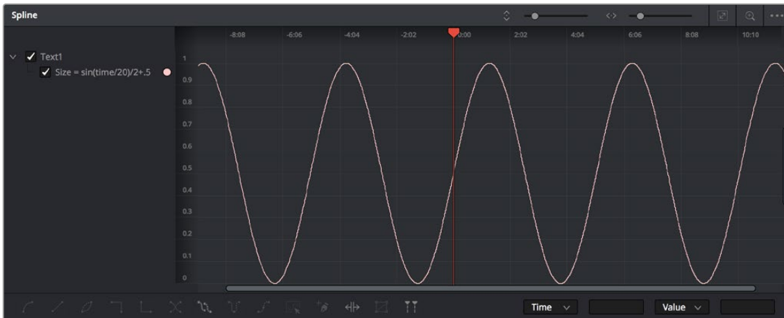
A sine wave in the Spline Editor, generated by the expression used for Text1: Size
