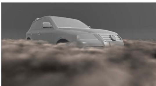
Without a bounding mesh to generate Position values, the fog fills in the background incorrectly
