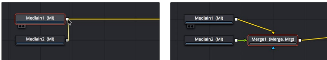
Dragging a connection from a disconnected node to another node's output (left), and dropping it to create a Merge node composite (right).
