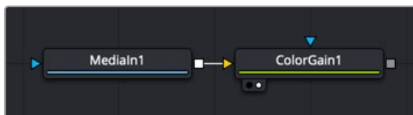
A Color Gain node applied to a MediaIn1 node
