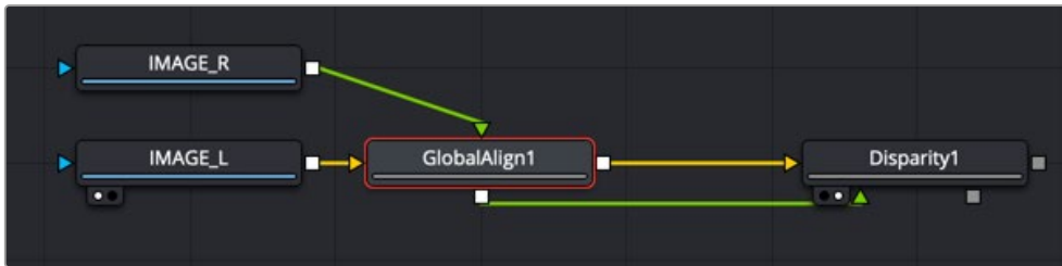
A Global Align node used to manually correct left and right eye discrepancies
