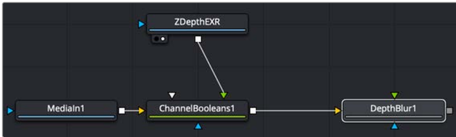
Depth Blur is applied to the beauty image based on a Z depth channel
