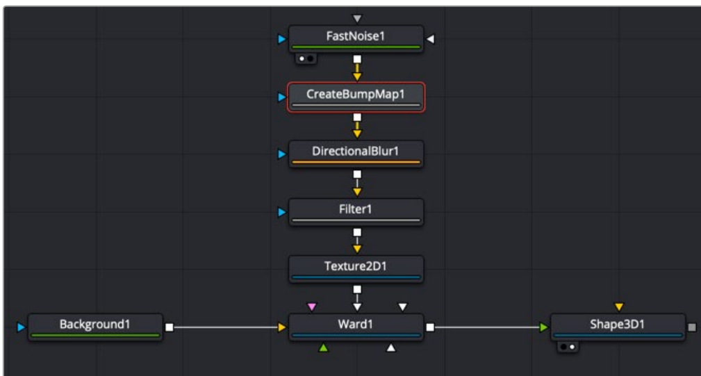
A Create Bump Map node produces a bump map as an RGB image for further image processing
