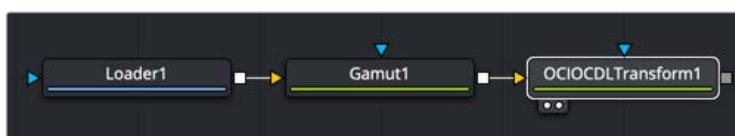
A OCIO CDL Transform node applied to a Loader node after a Gamut conversion to linear in Fusion Studio
