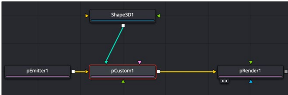
A pCustom node using a Shape 3D node as the region where the custom event occurs
