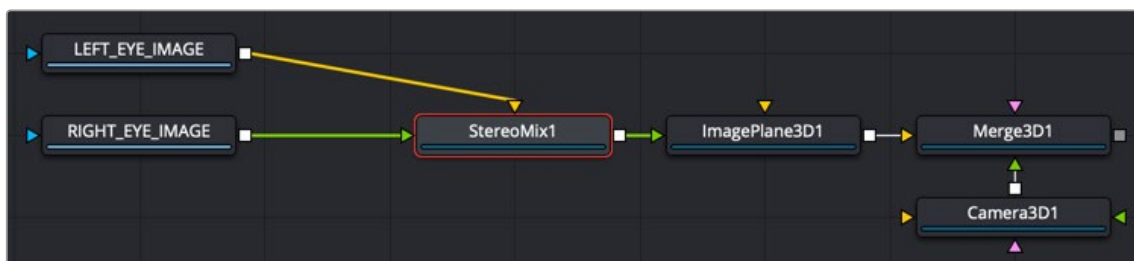
A Stereo Mix node used to combine left and right images into a single stereo material
