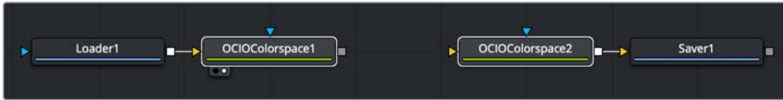
An OCIO Color Space node applied to a Loader node and a Saver node in Fusion Studio
