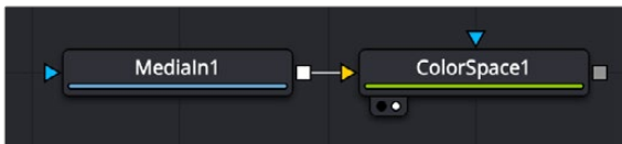
A Color Space node applies a conversion to a MediaIn1 node
