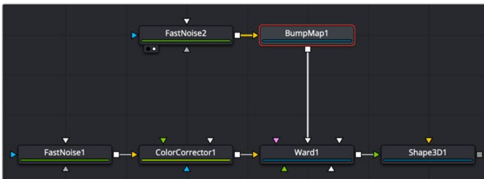
A Bump Map is connected to the Bump Map material input on a material node.
