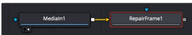
A Repair Frame node set up to analyze a MediaIn node using internal optical flow analysis.
