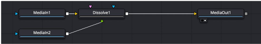
A typical dissolve node structure in Fusion
