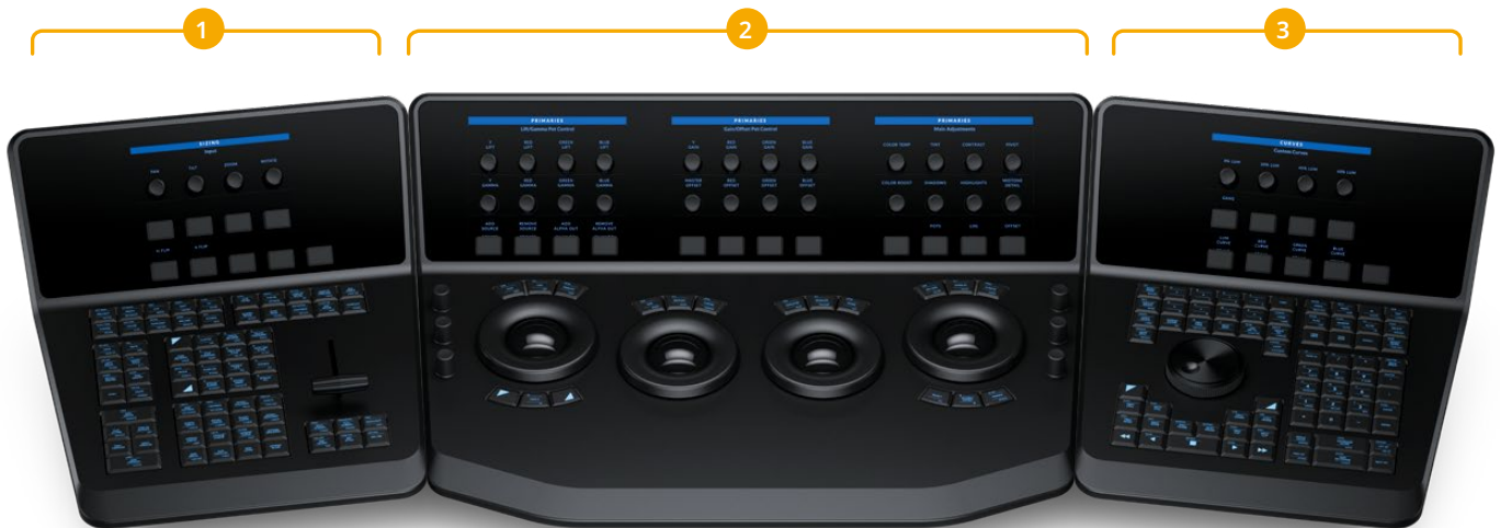
1. T-bar panel 2. Trackball panel 3. Search Dial panel
