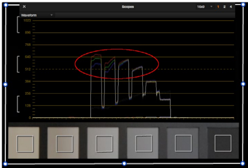
Poorly lit chart with irregularly topped waveforms
