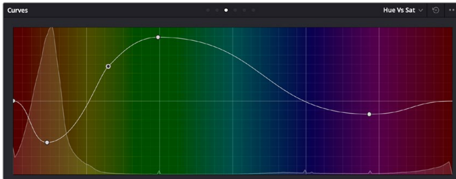
The histogram appearing underneath the Hue vs Sat curve plots all saturation levels at each value of hue
