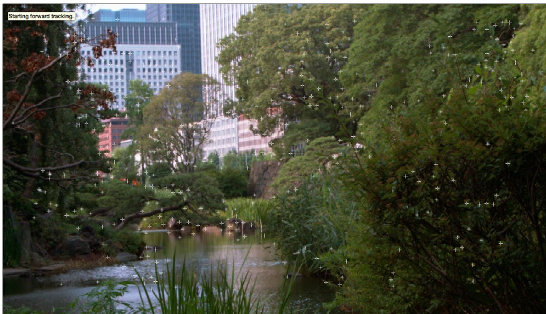
Multiple tracking points are automatically placed to analyze the motion of the image for stabilization
