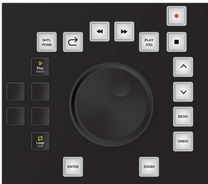
Shuttle/jog wheel with Fixed keys and default Play menu and Loop picture keys
