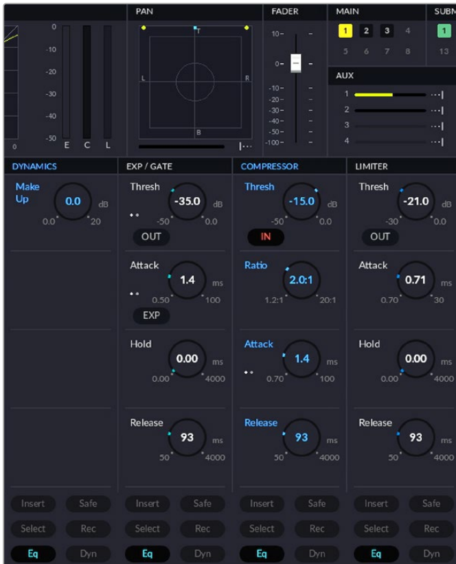
Compressor control set visual feedback in optional HDMI monitor. All Focus mode dynamics parameters grouped together in one section of the HDMI data screen. The active dynamics controls are highlighted in blue.
