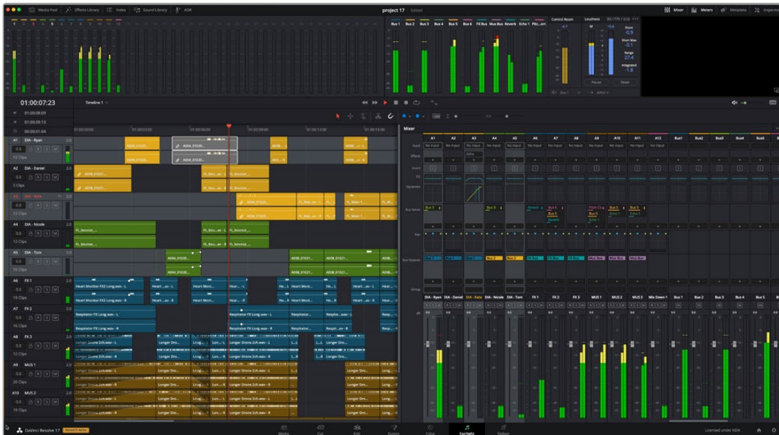
The Fairlight Timeline and Mixer showing the same track selection, A1, A3, and A5, with A3 as the active track.
