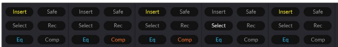
In-line Channel Extension buttons displayed at the bottom of the Channel LCD
