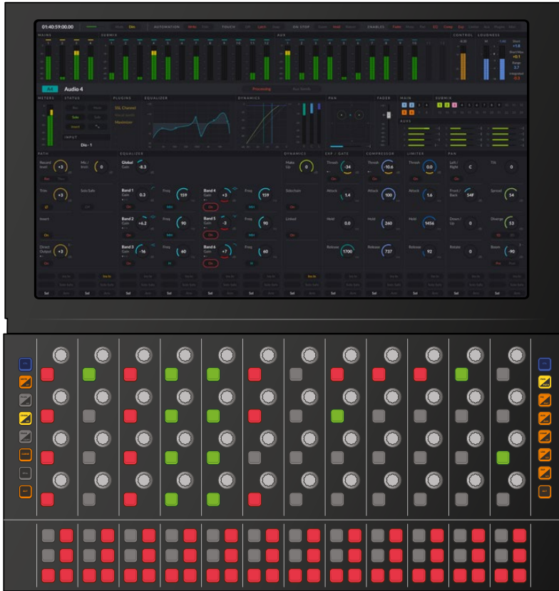
Channel display mode showing alternating colored buttons to separate parameter groups and unlit buttons where there are no matching on-screen parameters
