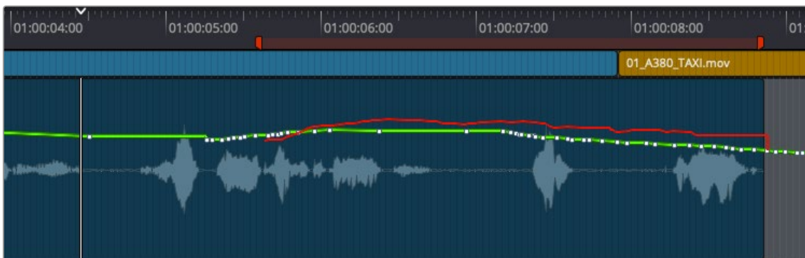
Active Range shown in the ruler with red bar; Automation data being written within the range..
