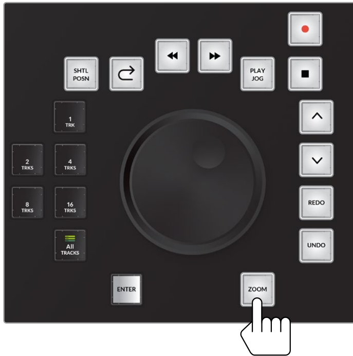
Zoom soft menu picture keys, including 1 Track, 2 Tracks, 4 Tracks, 8 Tracks, 16 Tracks, and All Tracks
