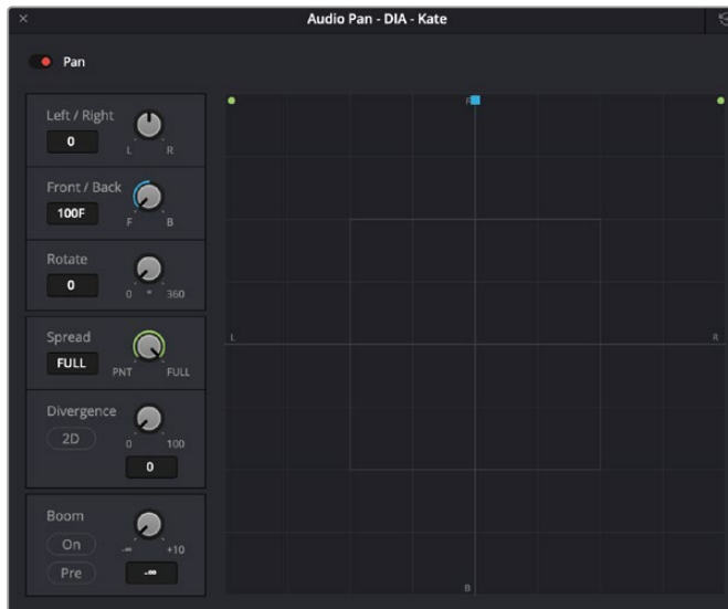
Pan control set mapping includes all parameters in the Fairlight Pan window.
