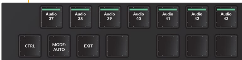
Auto Fader Bank mapping action keys in the lower left corner of the picture keyboard
