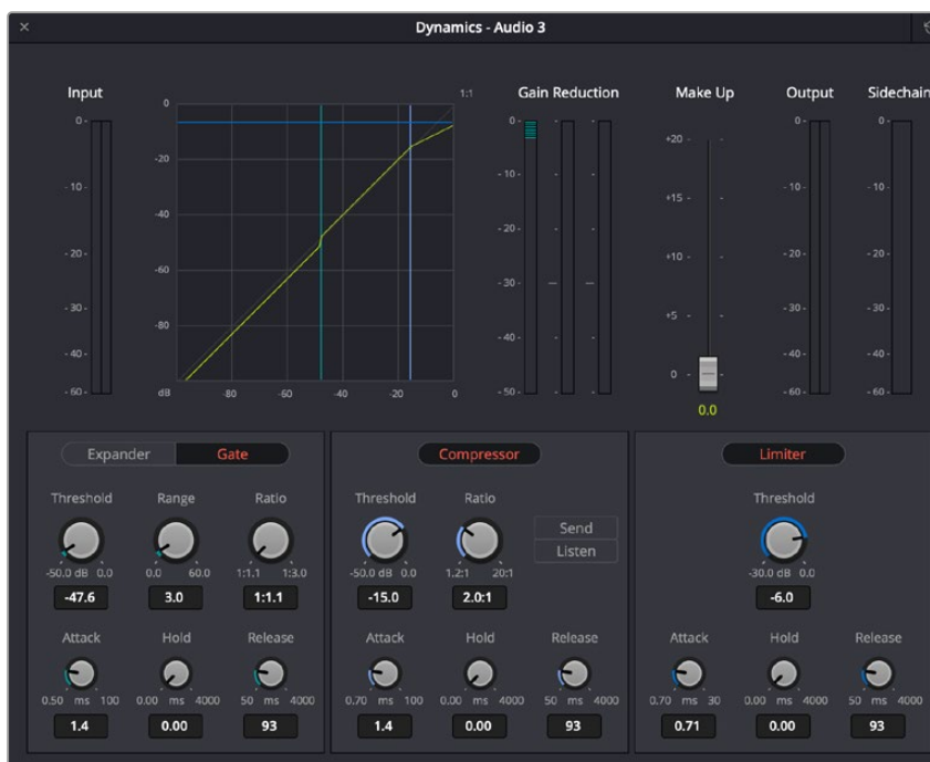
The channel strip Dynamics control window
