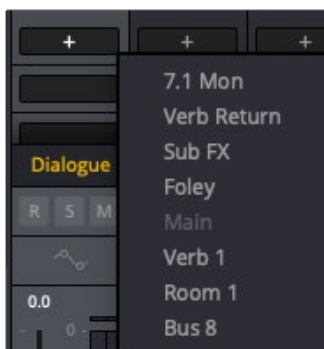
Bus routing drop-down menu on a channel strip
