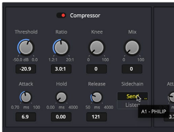
Enabling sidechain Send in the Compressor of a track with dialogue
