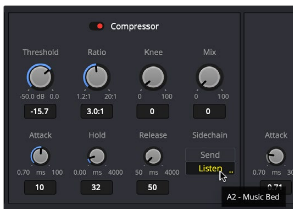
Enabling side chain Listen on the Compressor assigned to a music track
