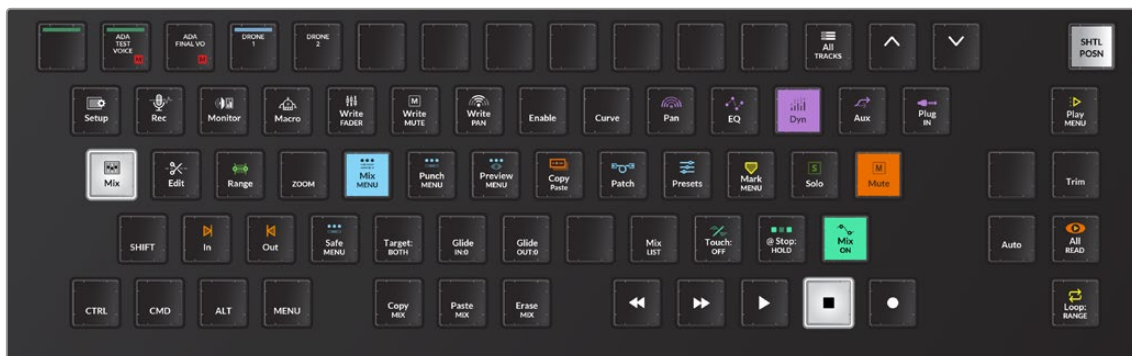
Mix Mode keys with Mix On latched; the automation toolset showing and Copy/Paste unlatched
