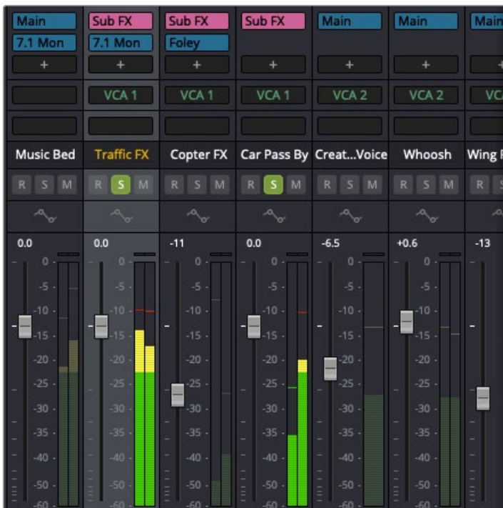
Pre-fader metering with light shaded meters on non-soloed tracks
