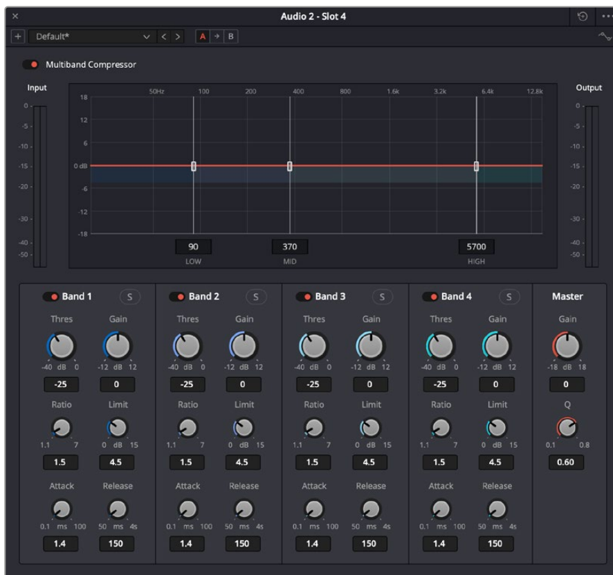
The default setting of the Multiband Compressor
