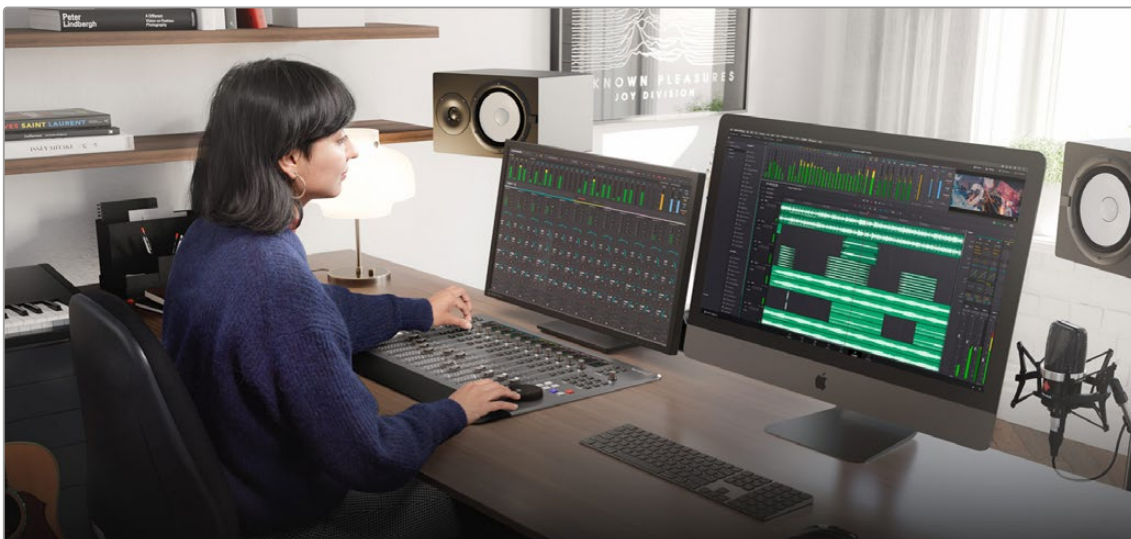
Fairlight Desktop Console connected to a second monitor via HDMI with nearby computer screen to display the DaVinci Resolve interface and enhanced channel-based visual feedback from the console on the HDMI screen
