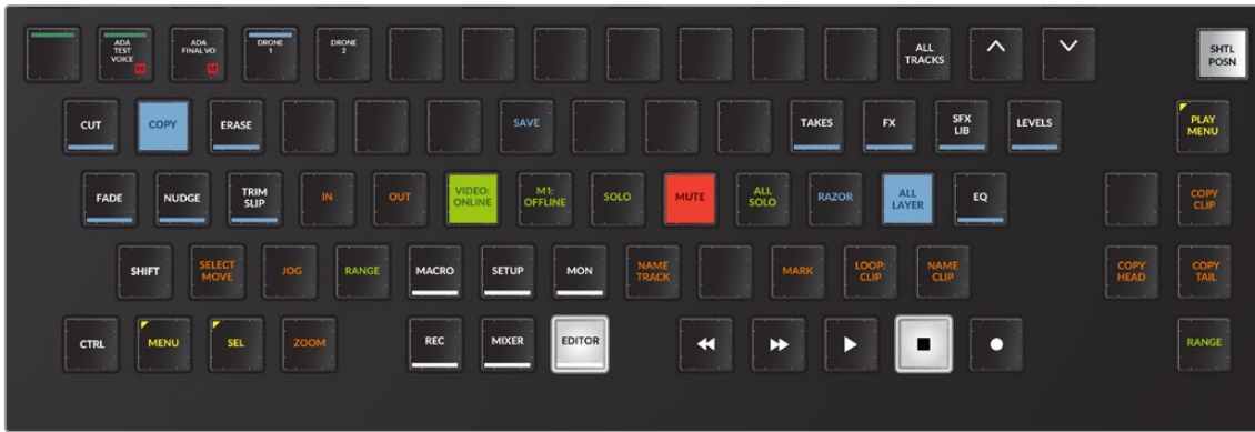
Alternate Editor toolset with Copy latched and Copy action keys available near the jog wheel
