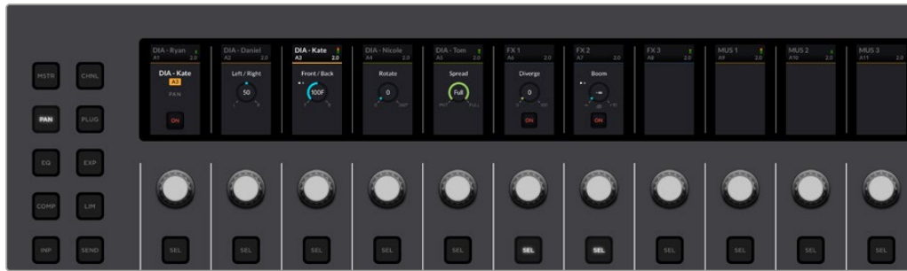
Pan control set mapping includes all parameters in the Fairlight Pan window.
