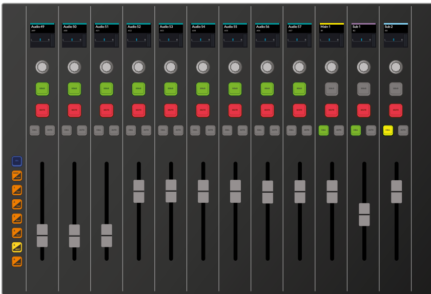
Bank/Flip Bank Display Button momentarily held to display the buses within the active track; these buses (in the right 3 channels) can be easily identified by the green Call buttons
