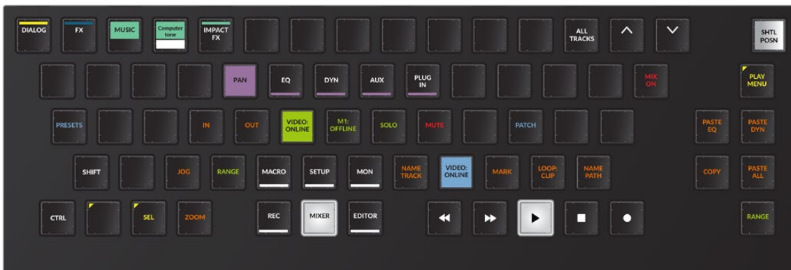
Alternate Mixer toolset with Mix On unlatched, Copy/Paste latched, and Copy/Paste keys available near the jog wheel
