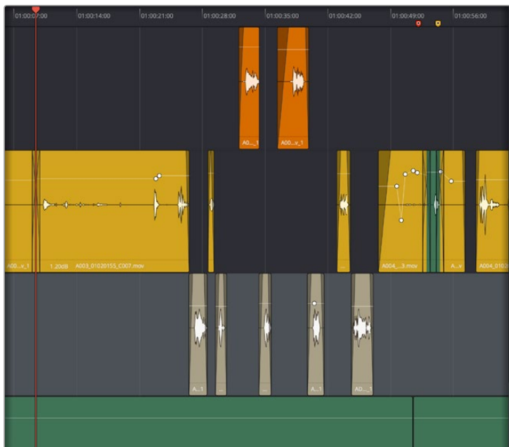
All of the highlighted clips have been faded according to the Batch Fades window.
